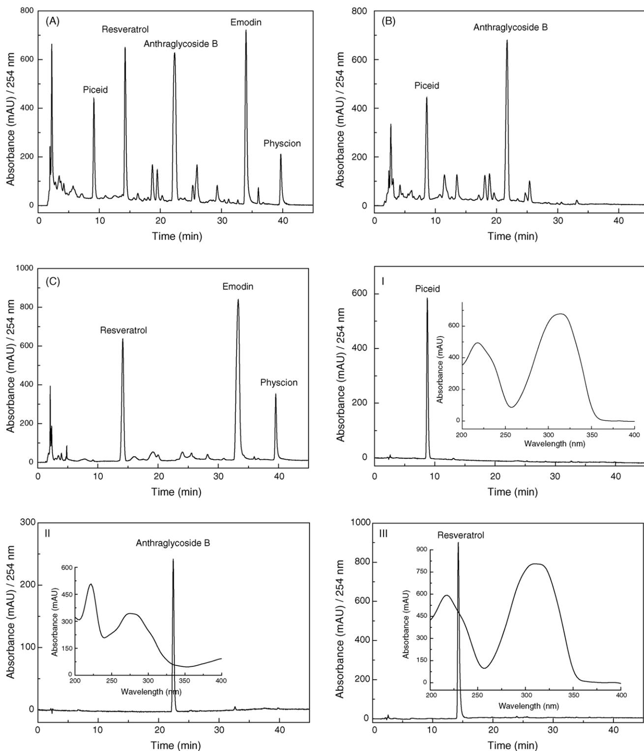
Fig. 2. HPLC chromatograms of crude extract (A), sample 1 (B), sample 2 (C) from *P. cuspidatum*, and HSCCC peak fractions (I–V), Column: SPHERIGEL ODS C<sub>18</sub> column (250 mm × 4.6 mm I.D., 10 μm); mobile phase: methanol–water (methanol: 0–15 min, 30–50%; 15–35 min, 50–90%; 35–45 min, 95%); flow rate: 1.0 ml min<sup>-1</sup>; detection wavelength: 254 nm.
