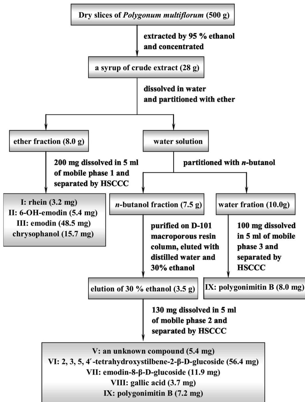
Fig. 2. Roadmap of extraction and separation. Mobile phase 1: the lower phase of *n*-hexane–ethyl acetate–methanol–water (3:7:5:5, v/v/v/v); mobile phase 2: the lower phase of ethyl acetate–methanol–water (50:1:50, v/v/v); mobile phase 3: the lower phase of ethyl acetate–*n*-butanol–water (20:1:20, v/v/v).
