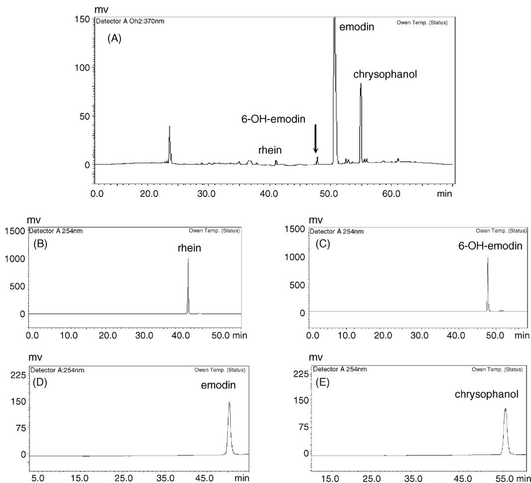
Fig. 4. HPLC chromatograms of two fractions of ether (A) and *n*-butanol (F) from *Polygonum multiflorum* Thunb. and HSCCC peak fractions of them (B–E, G–H) Column: Shimadzu VP-ODS (150 mm × 4.6 mm I.D., 5 μm); mobile phase (A–E): methanol–water (methanol: 5% to 100% in 60 min); flow rate: 1.2 ml/min; detection wavelength: 254 nm; mobile phase (F–H): acetonitrile–water (acetonitrile: 1% to 100% in 45 min); flow rate: 0.8 ml/min; detection wavelength: 254 nm.
