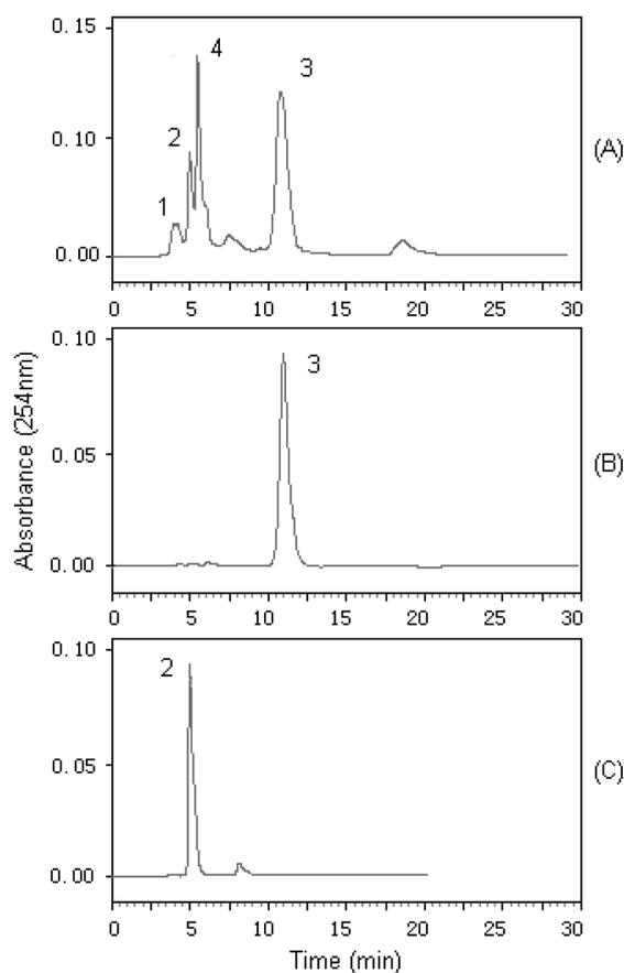
**Figure 3.** Results of HPLC analyses of the crude sample of *Prunus armeniaca* L. and its HSCCC fraction. Column: Shim-Pack CLC-ODS C<sub>18</sub> column (250 mm × 6 mm I.D.); mobile phase: acetonitrile–water (17 : 83); flow-rate: 0.6 ml/min; UV detector: 254 nm. (A) The crude sample; (B) HSCCC fraction from Peak 3; (C) HSCCC fraction from Peak 2 (Fig. 2).
