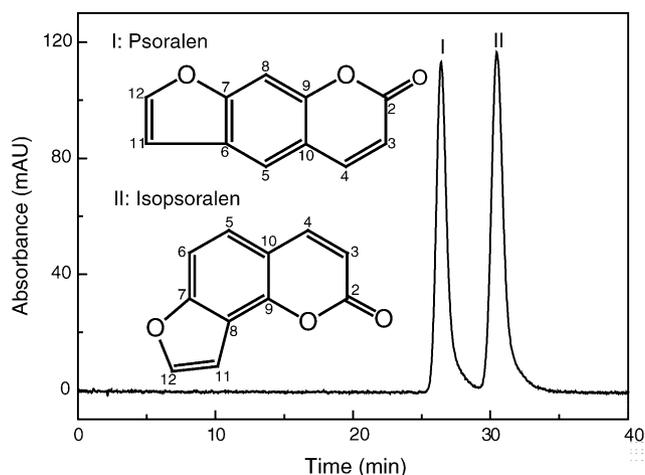
Fig. 1. HPLC chromatograms of crude extract from *P. corylifolia*. Conditions: column, reversed-phase YWG C<sub>18</sub> column (200 mm × 4.6 mm i.d., 10 μm); mobile phase, methanol–water (40:60, v/v); flow rate, 1.0 ml min<sup>-1</sup>; detection wavelength, 254 nm.
