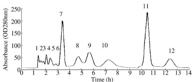
Fig. 1. Chromatogram of crude sample of *S. miltiorrhiza* Bunge from Hebei province by HSCCC separation. Conditions: column: multilayer coil of 2.6 mm i.d. tube with a total capacity of 300 mL; rotary speed: 900 rpm; stationary phase: the upper phase of solvent system A; mobile phase: 0–470 min, the lower phase of solvent system A and after 470 min, the lower phase of solvent system B; flow-rate: 2 mL/min; detection at 280 nm; sample size: 100 mg; retention of stationary phase: 78.8%.
